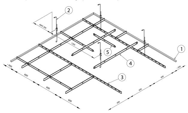
\*Verify the interaxe according to the load on m<sup>2</sup>.
